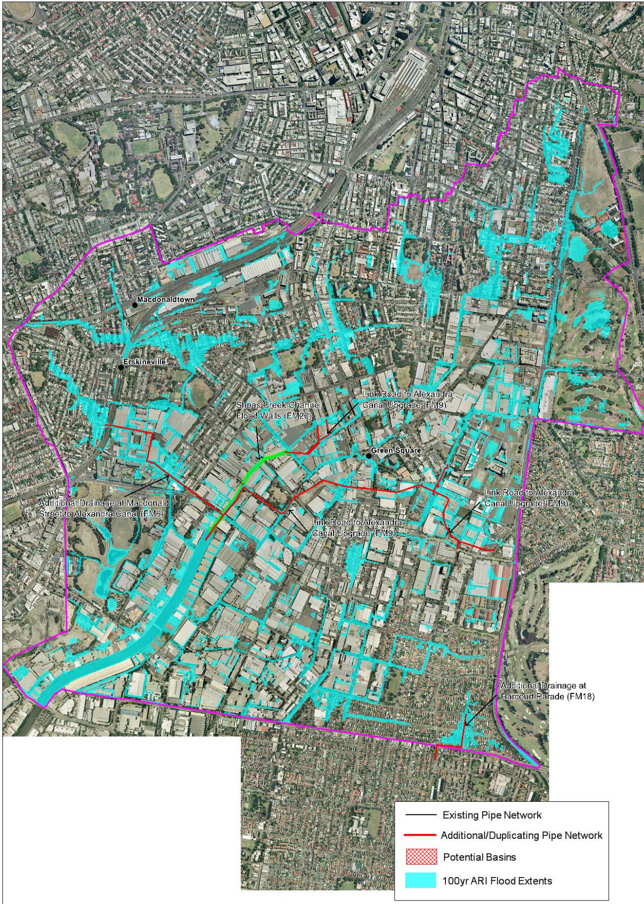
Figure 5-1 Recommended Structural Measures
